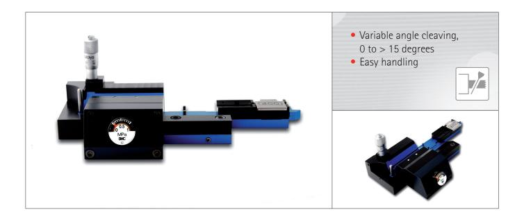
An angle cleaving option is now available for the NYFORS AutoCleaver LDF $^{\text{TM}}$ . Designed as a rotary clamp, the angle cleaving unit produces accurately angled cleaves of up to 15 degrees on large diameter fibers with a coating diameter from 250 to 1000  $\mu$ m.
