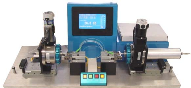
fig. 5 Measurement setup for the orientation of PM components using the cross polarizers method.
