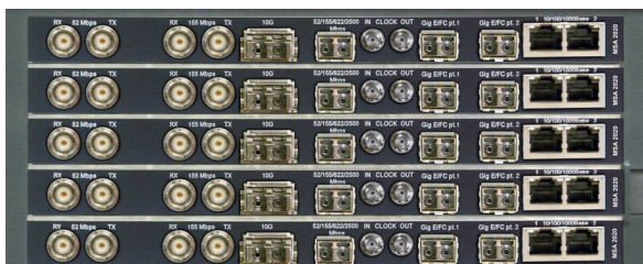
Figure H: NIC Plus Configured with Five MSA-series Modules
