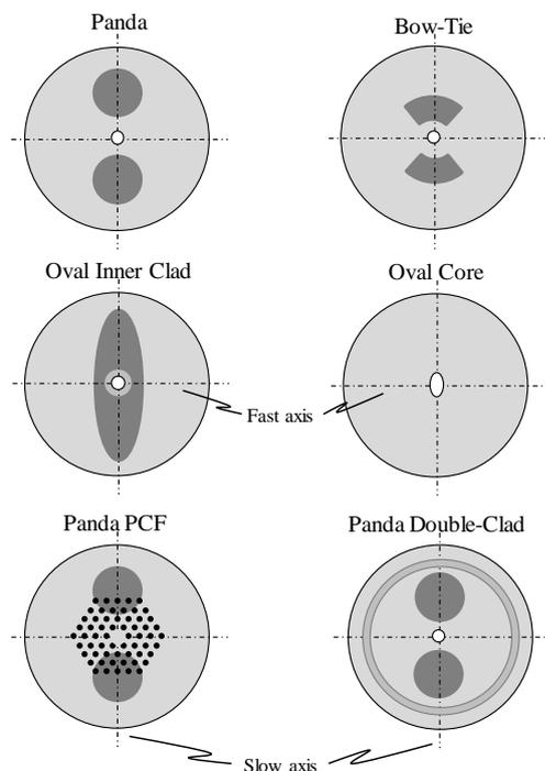
**Figure 4. Examples of schematic cross-sections of a few PM fiber structures. The dark features represent the stress elements used to induce birefringence. Fast axes are oriented horizontally while the slow ones are vertical.**
