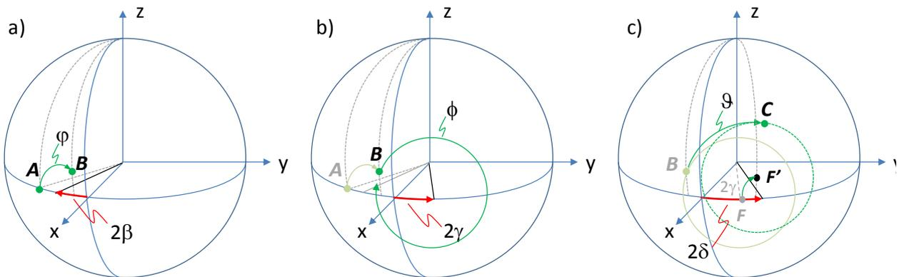
Figure 5. Evolution on the Poincaré sphere of a SoP during the propagation through three mutually misaligned waveplates. The first (a) and the last (c) waveplate impose a fix delay ( $\varphi$  and  $\vartheta$ , respectively) while the phase  $\phi$  of the central waveplate (b) is swept over  $2\pi$ . More details in the text.
