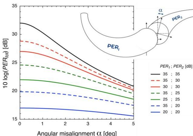
**Figure 9. Total polarization performance of two PM elements in series with selected PER values vs. the angular mismatch  $\alpha$ . Solid lines represent fibers with the same PER, dotted lined show examples with a fix fiber ( $PER_1=35$  dB) connected to fibers with decreasing  $PER_2$ . Note that the PER values are expressed on a logarithmic scale.**
