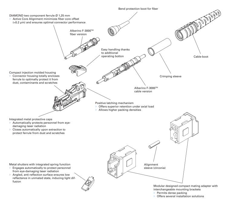
NOTE As standard, Diamond uses colored connector bodies, cable boots and mating adapter housings to identify the fiber type (SM or MM 50/62.5µm) and ferrule polish (PC or APC).
