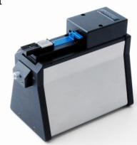
THE CLEAVEMETER 3D™ is a non-contact interferometer designed for inspecting the end-faces of cleaved or polished optical fibers with cladding diameters of 125 µm to 1200 µm. It gives immediate and precise information on important end-face properties such as flatness, perpendicularity, hackles and dust. Based on the NYFORS CLEAVEMETER 2™ design, in addition to producing sharp fringe patterns it also generates three-dimensional images of the cleaved fiber end.
