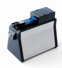
The CLEAVEMETER  $2^{\text{TM}}$  is a non-contact interferometer designed for inspecting the end-faces of cleaved or polished optical fibers with cladding diameters of 125  $\mu$ m to 1200  $\mu$ m. It gives immediate information on important end-face properties such as flatness, perpendicularity, hackles and dust. Sampling tests as well as continuous process documentation can be carried out both easily and quickly, making this an ideal instrument for cleaver inspection and optimisation.
